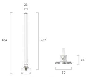
Main Unit Dimension : 457 \* 22mm(L x W) Including bracket : 484 \* 70 \* 35mm(L x W x H) Weight : 156g / 216.5g ( Including bracket )
