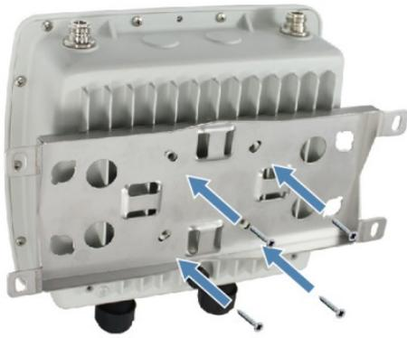
**Instructions:** Use the provided screws to secure the mounting bracket on the back of OW-400-A2. The bracket can be attached two different ways.
