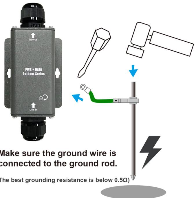
**Make sure the ground wire is connected to the ground rod.**
