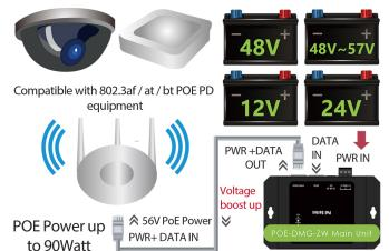
Main application method of Boost adapter to POE Injector
