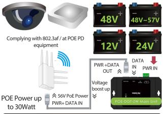
Main application method of Boost adapter to POE Injector
