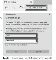
If you can't to login to DT-300N v2 WEB management interface, please reset default the DT-300N v2 to factory default ( Press the "reset" button for  ${\bf 10}{\text{-}}{\bf 15}$ seconds located on rear panel then release it and DT-300N v2 will automatically restart and restore to default settings. ) then try to login again and make sure there is no others network devices use the same IP address with DT-300N v2.
