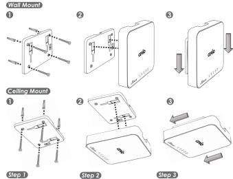
Position the Mounting Bracket in the desired location.Use the screws and anchors in the mounting kit to secure
