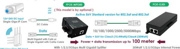
12V~24V 11ac/11ax DC Input Single Giga or Multi-Giga WiFi Access Point 30Watt 1/2.5/5Gbps Internal Power Multi Gigabit PoE+ Injector
