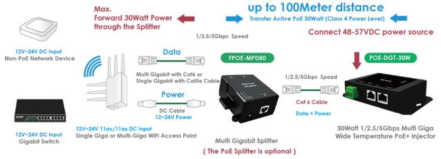
\* The gigabit splitter allows a non compliant device to upgrade to PoE. It is used to deploy remote non-PoE devices with no nearby AC outlets.
