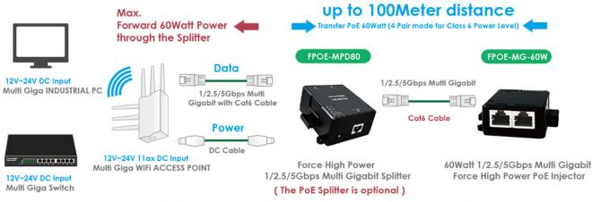
\* The force high power splitter allows a non compliant device to upgrade to PoE, It is used to deploy remote non-PoE devices with no nearby AC outlets.
