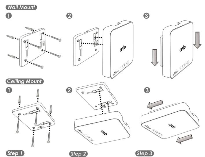
Position the Mounting Bracket in the desired location.Use the screws and anchors in the mounting kit to secure the Bracket into position.
