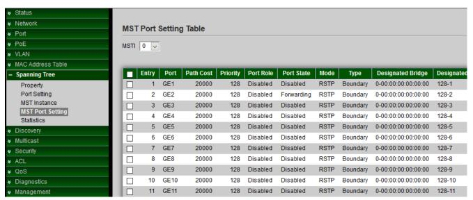
MST Port Settings is used to configure the port MSTP settings for every MST instance. It is also used to view statistics that have been learned from the protocol.
