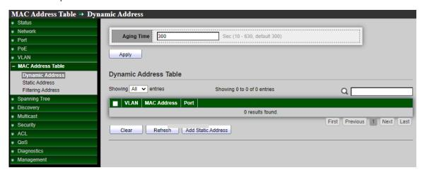
When administrator select checkbox MACs address and click "Add Static Address" button then selected MAC address will move to "Static Address" function.
