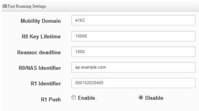
Mobility Domain: MDID is used to indicate a group of APs (within an ESS, i.e., sharing the same SSID) between which a STA can use Fast BSS Transition.
