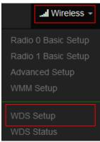
When the WDS function is enabled, it can be set to use Radio 0 (2.4G) for WDS or Radio 1 (5G) for WDS, etc., and a maximum of 24 groups can be set up to bridge to 2.4G + 5G + 5G. In WDS The function supports VLAN tag transmission. If there is a tag set in the network domain, WDS can bring multiple groups of tags to another bridge endpoint.
