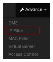
Can allow or deny filter ingress or egress packets from specific source and/or to destination IP address on wired (LAN) or Wireless (WAN) ports. Filter rules could be used to filter unicast or multicast packets on different protocols as shown in the IP Filter Setup. Important to note that IP filter rules has precedence over Virtual server rules. Total of 20 rules maximum allowed in the IP Filter List. All rules can be edited or removed from the List.
