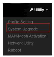
Firmware is the main software image that system needs to respond to requests and to manage real time operations. Firmware upgrades are sometimes required to include new features or bugs fix. It takes around 2 minutes to upgrade due to complexity of firmware. To upgrade system firmware, click Browse button to locate the new firmware, and then click Upgrade button to upgrade.
