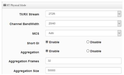
TX/RX Stream: Build in 2.4GHz 2 antennas and support 2TX/2RX streams. Administrator can select 1 or 2 TX/RX. The default is 2TX/2RX.
