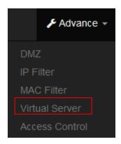
The "Virtual Server" can also referred to as "Port Forward" as well and used interchangeably. Resources in the network can be exposed to the Internet users in a controlled manner including on-line gaming, video conferencing or others via Virtual Server setup. Don't repeat ports' usage to avoid confusion.
