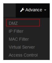
DMZ is commonly work with the NAT functionality as an alternative of Virtual Server(Port Forwarding) while wanting all ports of DMZ host visible to Internet users. Virtual Server rules have precedence over the DMZ rule. In order to use a range of ports available to access to different internal hosts Virtual Server rules are needed.
