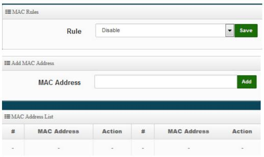
Rule: Select the desired access control type from the drop-down list; the options are Disable, Allow or Reject.
