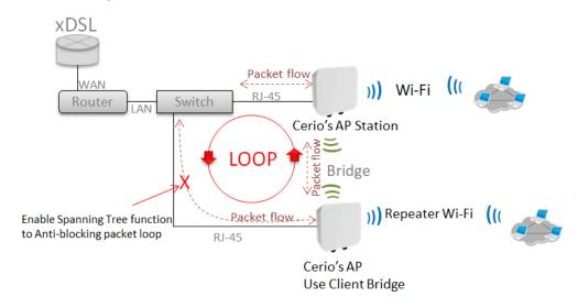
➤ DHCP Forward: When the AP Mode device and Client Bridge AP are linked, and DHCP Service is "Enabled", the Client Bridge AP must also enable DHCP Forward to allow connecting clients to receive the IP Address from the source AP (AP Mode Device). By default, DHCP Forward is disabled in Client Bridge devices. This function must be enabled to allow clients connecting to the Client Bridge device to receive IP Addresses from the source AP.
