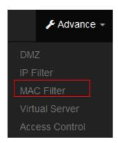
Allows creating MAC filter rules to allow or deny unicast or multicast packets from limited number of MAC addresses. Important and must note. That MAC filter rules have precedence over IP Filter rules.
