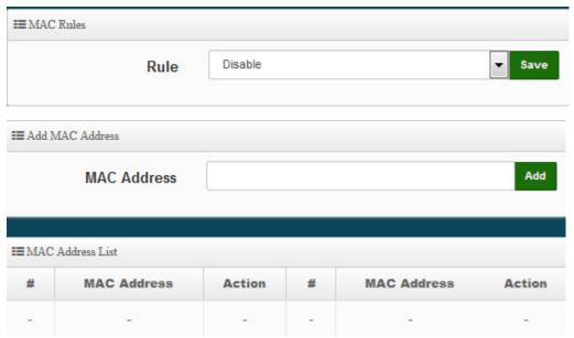
> Rule: Select the desired access control type from the drop-down list; the options are Disable, Allow or Reject.
