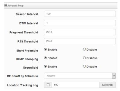
Beacon Interval: Beacon Interval is in the range of 40~3500 and set in unit of millisecond. The default value is 100 msec.
