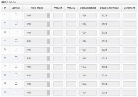
QoS Rule List: Administrator can set bandwidth limit by IP/MASK, IP Range, Port(Service), SIP, RTP/RTSP, WEB protocol, each VLAN can set 10 bandwidth management rule.
