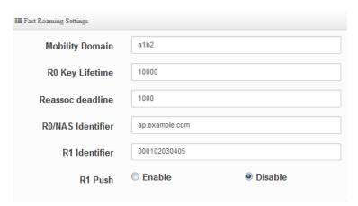
Mobility Domain: MDID is used to indicate a group of APs (within an ESS, i.e., sharing the same SSID) between which a STA can use Fast BSS Transition.
