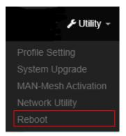
This function allows user to restart system with existing or most current settings when changes are made. Click **Reboot** button to proceed and take around three minutes to complete.
