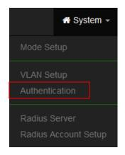
When enable web authentication function, please does make the Access Point can be connected to gateway. Please refer to VLAN Setup. If the gateway IP address is set error address then web login page can't display
