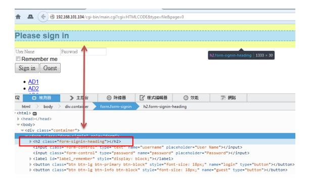
Add <style> .form-signin-heading {display: none;} </ style> in the head to hide the description "Please Sign in" as shown in the figure below, and find the Please Sign in word disappeared, and so on.
