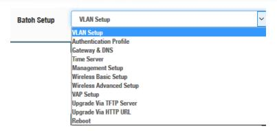
VLAN Setup: Administrator can set VLAN Tag, IP address and Wi-Fi on/off for the managed APs.
