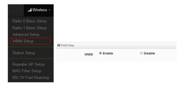
As an Example, time-sensitive Voice & Video, and multimedia are given effectively higher priority for transmission (lower wait times for channel access), while other applications and traditional IP data which are less time-sensitive but often more data-intensive are expected to tolerate longer wait times.
