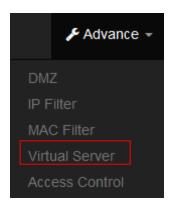
The "Virtual Server" can also referred to as "Port Forward" as well and used interchangeably. Resources in the network can be exposed to the Internet users in a controlled manner including on-line gaming, video conferencing or others via Virtual Server setup. Don't repeat ports' usage to avoid confusion.
