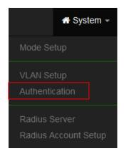
When enable web authentication function, please does make the Access Point can be connected to gateway. Please refer to VLAN Setup. If the gateway IP address is set error address then web login page can't display
