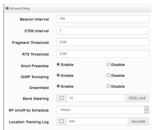
Beacon Interval: Beacon Interval is in the range of 40~3500 and set in unit of millisecond. The default value is 100 msec.
