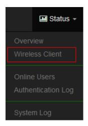
The page can be display Wireless user information link to access point. Administrator can monitor MAC address / rate and RSSI for the wireless users. (In addition to CAP mode)
