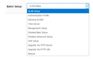
VLAN Setup: Administrator can set VLAN Tag, IP address and Wi-Fi on/off for the managed APs.
