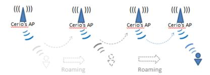
The dual band Access Point supports 802.11r/802.11k function for 2.4G and 5G radio. 802.11r, which is the IEEE standard for fast roaming, introduces a new concept of roaming where the initial handshake with the new AP is done even before the client roams to the target AP.
