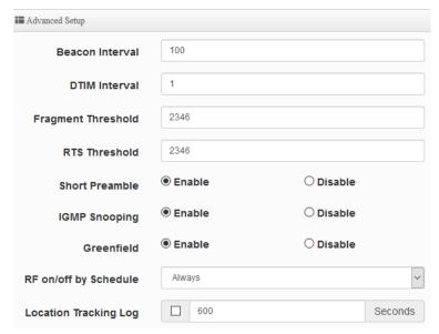
Beacon Interval: Beacon Interval is in the range of 40~3500 and set in unit of millisecond. The default value is 100 msec.
