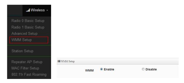
As an Example, time-sensitive Voice & Video, and multimedia are given effectively higher priority for transmission (lower wait times for channel access), while other applications and traditional IP data which are less time-sensitive but often more data-intensive are expected to tolerate longer wait times.
