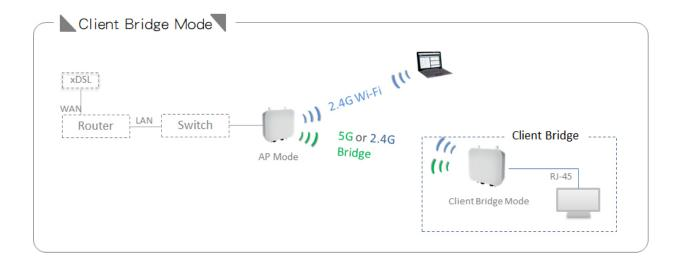
Note: If Client Bridge used 5GHz connection to AP station then Repeater AP only use 2.4GHz.
