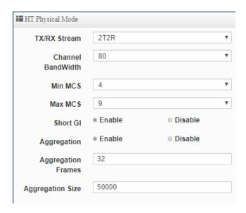
TX/RX Stream: supporting 2TX/2RX streams. Administrator can select 1 or 2 TX/RX. The default is 2TX/2RX.
