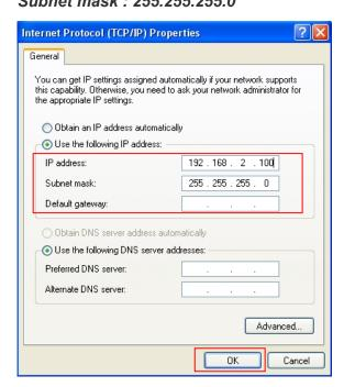
Click "OK" completion set up IP address
