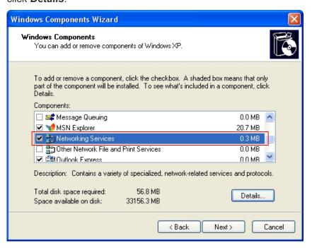
ii. In the "Networking Services" window, ensure that the "Internet Gateway Device" and "UPnP User Interface" options are checked. If they are not, check it to enable them, as shown below, and click OK to continue.
