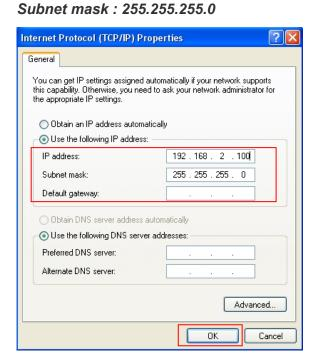
Click "OK" completion set up IP address
