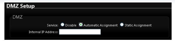
Static Assignment: Enter external and internal IP address of DMZ host. The function only external IP to Internal IP address
