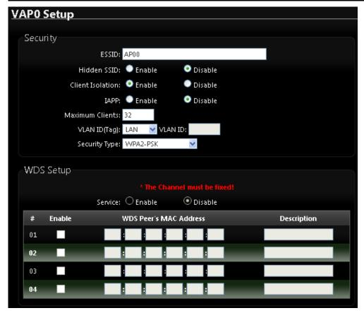
ESSID: Extended Service Set ID indicates the SSID which the clients used to connect to the VAP. ESSID will determine the service type of a client which is assigned to the specified VAP.
