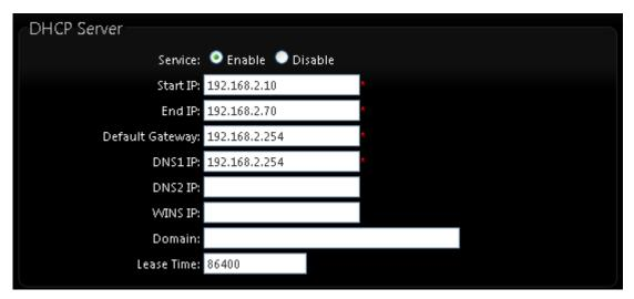
DHCP: Check *Enable* button to activate this function or *Disable* to deactivate this service.
