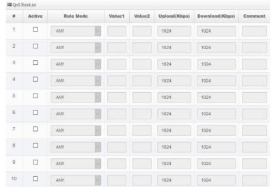
QoS Rule List: Administrator can set bandwidth limit by IP/MASK, IP Range, Port(Service), SIP, RTP/RTSP, WEB protocol, each VLAN can set 10 bandwidth management rule.
