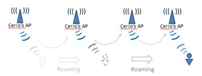
The dual band Access Point supports 802.11r/802.11k function for 2.4G and 5G radio. 802.11r, which is the IEEE standard for fast roaming, introduces a new concept of roaming where the initial handshake with the new AP is done even before the client roams to the target AP.
