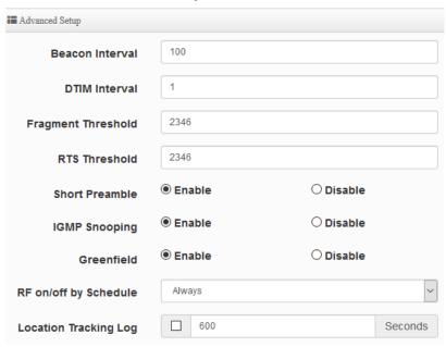
Beacon Interval: Beacon Interval is in the range of 40~3500 and set in unit of millisecond. The default value is 100 msec. Recommend use default.
