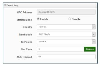
**Station Mode:** When administrator select enable mode will used this radio in the client bridge function. If select disable then used Repeater AP function.
