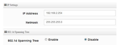
**IP Setup:** The administrator can manually setup the LAN IP address.
