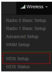
The administrator can create WDS Links for expanding wireless network via this page. When you enable "WDS" function in AP Mode both Wireless and Ethernet user can connect your local network at the same time through AP.
