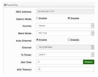
Station Mode: When administrator select enable mode will used this radio in the client bridge function. If select disable then used Repeater AP function.
