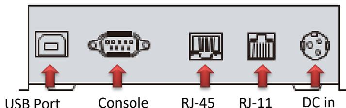
PS. Connect the controller only need to use RJ-45 and power.
