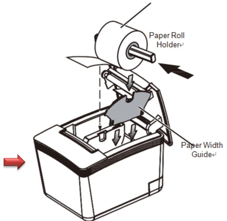
When using a paper roll in smaller width, install the Paper Width Guide first, and then install the paper roll with holder.
