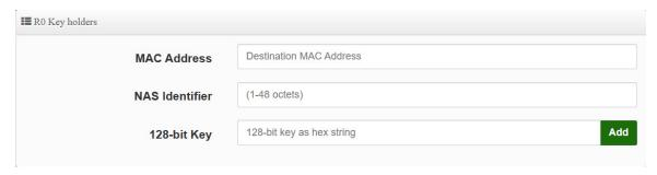
R0 Key holders: To enable roaming between multiple AP devices, AP1 must key in the MAC
