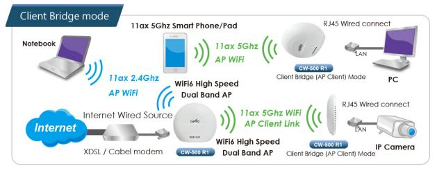
Note: If Client Bridge used 5GHz connection to AP station then Repeater AP only use 2.4GHz.
