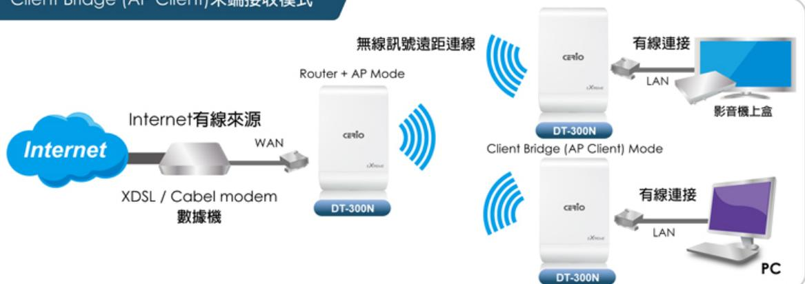
Client Bridge + Repeater AP 末端橋接模式+無線延伸中繼模式
