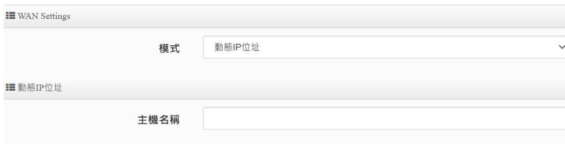
The screenshot shows the 'WAN Settings' section with the 'Mode' dropdown set to 'Dynamic IP Address'. Below it, the 'Dynamic IP Address' section is visible, showing a 'Host Name' input field.
