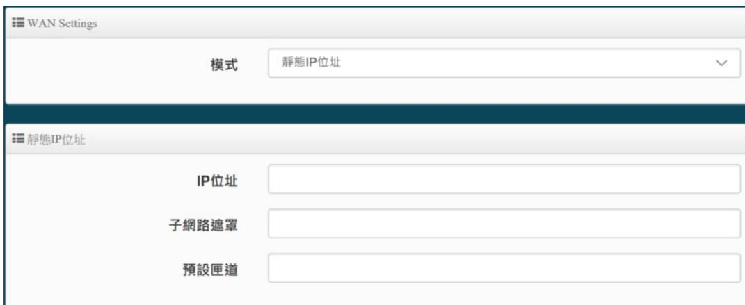
The screenshot shows the 'WAN Settings' interface. At the top, there is a 'Mode' dropdown menu set to 'Static IP Address'. Below this, there is a section titled 'Static IP Address' containing three input fields: 'IP Address', 'Subnet Mask', and 'Default Gateway'.
