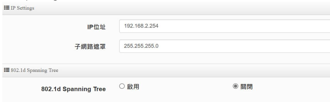
The screenshot shows two sections of the settings page. The top section is titled "IP Settings" and contains two input fields: "IP位址" (IP Address) with the value "192.168.2.254" and "子網路遮罩" (Subnet Mask) with the value "255.255.255.0". The bottom section is titled "802.1d Spanning Tree" and contains a label "802.1d Spanning Tree" followed by two radio buttons: "啟用" (Enabled) and "關閉" (Disabled). The "關閉" radio button is selected.
