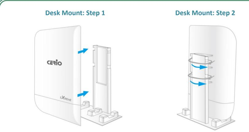
Click the DT-300N device securely onto the desktop mount through the blister mounting component on the back of the device. Use the self-locking cable ties to secure the DT-300N in place. Once mounted, simply place the device in desired location.
